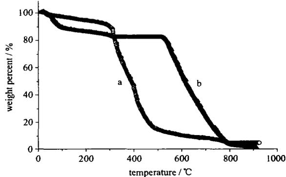
Fig. 3 Thermogravimetric analysis (TGA) of the SWCNTs
