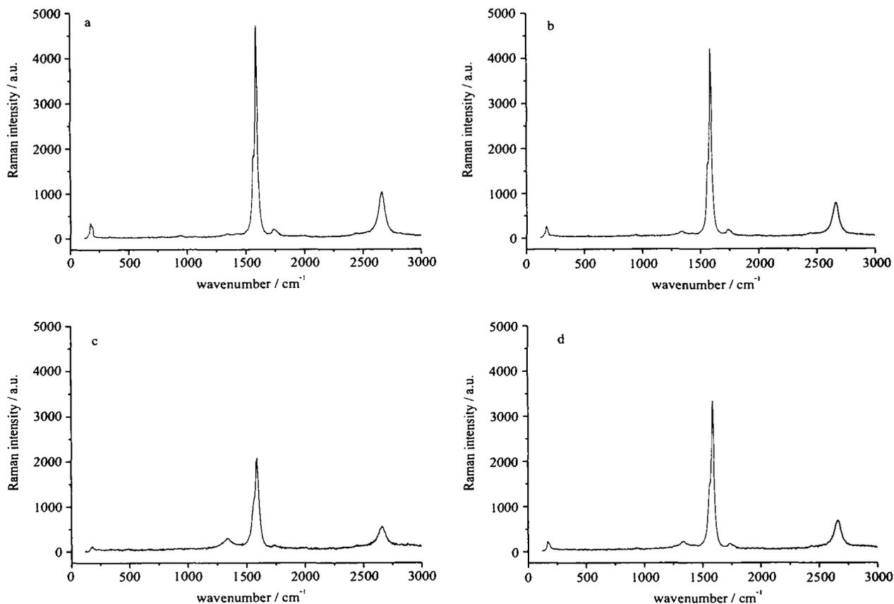
Fig. 2 Raman spectra of SWCNTs
