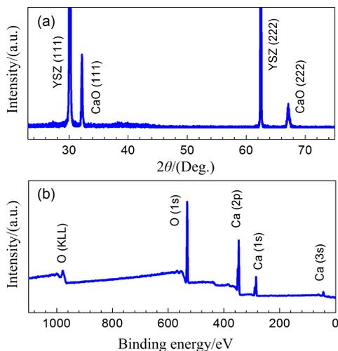
Fig. 1 (a) XRD  $2\theta$ - $\omega$  of CaO films grown on YSZ(111) substrates, and (b) XPS spectrum for CaO films with 320 nm
