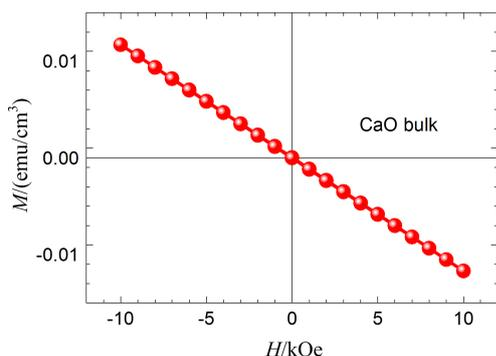
Fig. 2  $M$ - $H$  curve of the CaO bulk
