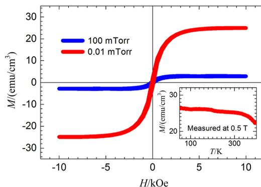
Fig. 3  $M$ - $H$  curves of CaO films for 100mTorr and 0.01mTorr. The inset in this figure shows the  $M$ - $T$  curve of CaO films grown at 0.01 mTorr
