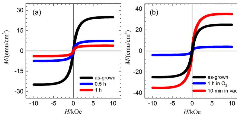
Fig. 4 (a)  $M$ - $H$  curves of CaO films and annealed in oxygen atmosphere for 0.5h and 1h and (b) in vacuum annealed at 400 °C and 0.01 mTorr after O<sub>2</sub> annealing
